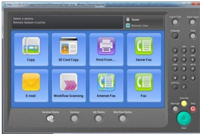
Screen shot of the ConnectKey Technology-enabled MFP user interface emulation displayed on a user PC. UI soft buttons and control panel hard buttons are fully operable using a local mouse and keyboard.
