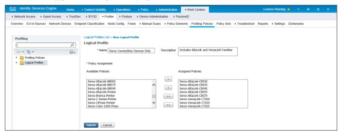
Figure 2: Logical Profile of "Xerox® ConnectKey® Devices Only", which groups all Xerox® AltaLink® and Xerox® VersaLink® devices and policies.
