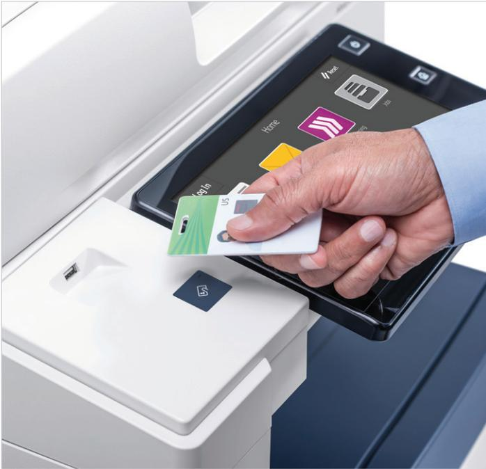
The 144k CAC/PIV is a version of the smart card. Users can be authenticated using two-factor identification to gain access to walkup services at the device.
