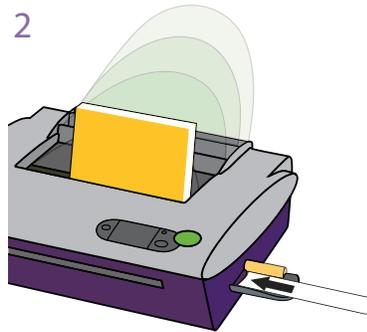
Machine automatically measures book thickness and requests a narrow, medium or wide strip. Insert binding strip.
