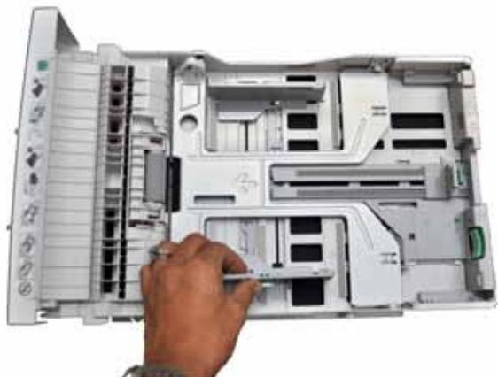
**Above and below:** In order to adjust the paper drawer to accommodate different paper sizes the user squeezes and slides these gray guides into place. BERTL found it easy to adjust the paper drawer.
