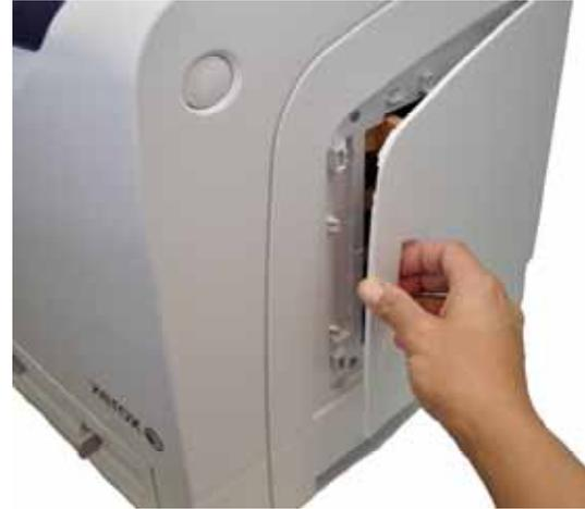
In order to replace the Xerox Phaser 6140N's toner cartridge the user must first open the devices side cover by pulling this panel door open.
