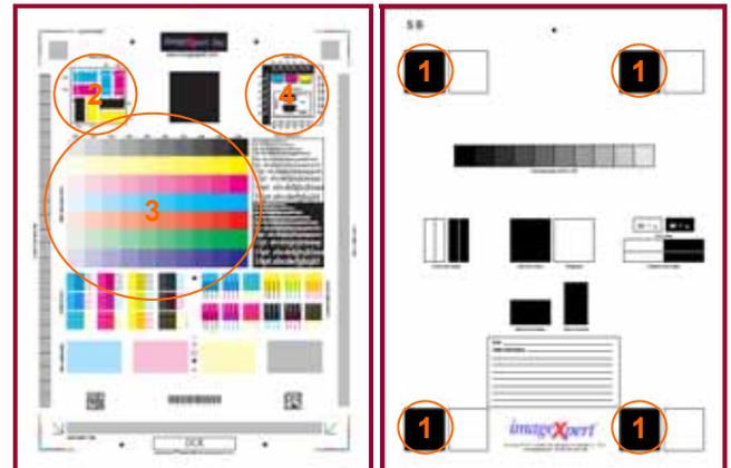
BERTL uses ImageExpert printer test targets for the evaluation of printed image quality. BERTL technicians' measure image density and evaluate the device's ability to produce a full range of halftones and various sizes of negative/positive text, dots and lines in each primary printing color (CYMK).
