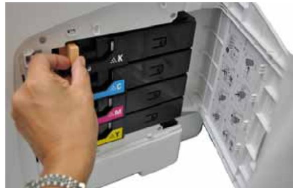
**Above and next page:** Once the door is open the user then unlocks the orange lever by sliding it to the right and pulling the toner cartridge out for replacement. Overall, BERTL found replacing the all four toner cartridges to be a simple process.
