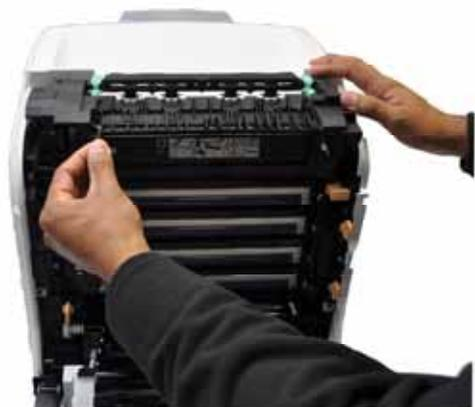
**Above and next column:** In order to replace the fuser unit the users presses this gray lever and slides the unit out for replacement.
