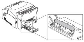
Rotate SIMM downward into connector until it snaps into place. Make sure both metal clips on connector are fastened and two pins on connector are pushed through the holes in the SIMM.
