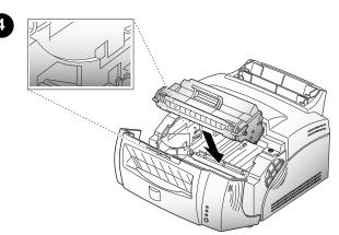
Unpack the new laser print cartridge by tearing open its packaging at the indicated notch, then carefully remove sealing tape from bottom of cartridge by pulling on sealing tape tab.
