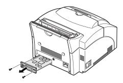
Be aware that control board is connected to inside of printer by two cables. Do not disconnect these cables.
