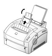
Fan stack of paper to loosen, then insert in MPF. Do not overload.
