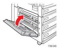
**4.** Pull out the tray specified on the control panel.
