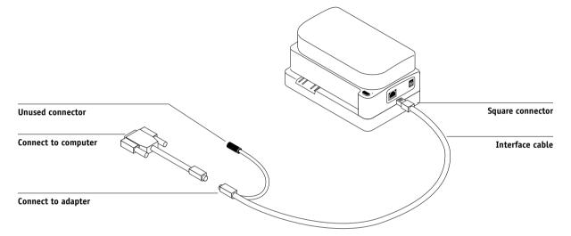
For a Mac OS computer, connect the 8-pin mini-DIN plug directly into the serial port of the computer.
