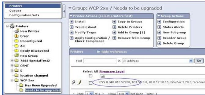
2. Select **Group Actions>Configuration>Membership Filter** and choose **Firmware Level Not Equal to {the device’s software level following the upgrade}**.
