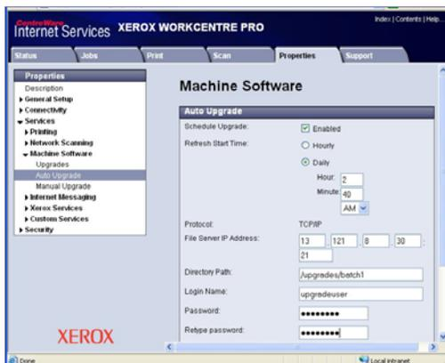
3. Check the **Enabled** box to enable the auto upgrade feature.
