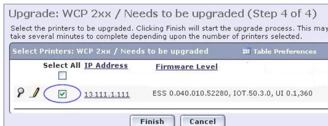
6. A list of the devices you identified appears. Check the box of each device to upgrade / patch / clone or check **Select All**. Click **Finish** to complete the Wizard and begin the process.
