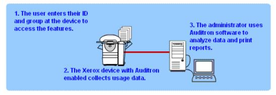
Refer to the documentation that came with your device for complete details about setup, configuration, and use of the Auditron.
