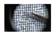
Xerox<sup>®</sup> Color C60/C70 Printer: 0.6 point font Xerox<sup>®</sup> MicroFont pictured with α pin.
