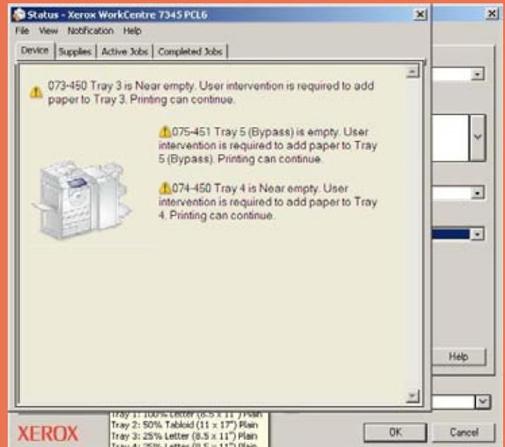
The "More Status" option's Device tab indicates current device status, while the Supplies tab (below) provides toner and paper status.
