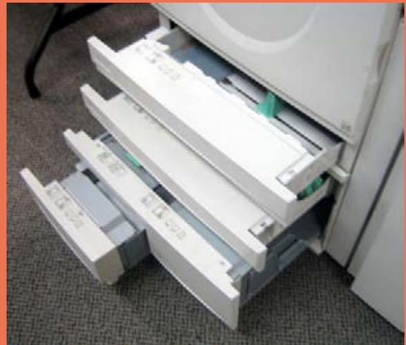
All of the WorkCentre 7345 paper sources can handle substrates as thick as 80-lb. cover stock.
