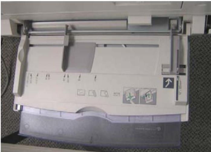
The WorkCentre 7345's 100-sheet bypass tray, which is located on the left side of the device.
