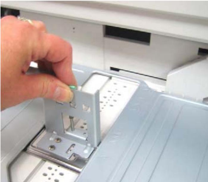
Adjusting the WorkCentre 7345's paper drawers is relatively easy; users squeeze the drawers' guides into place as shown above. There are no removable guides that must be removed and reinserted into the drawer.
