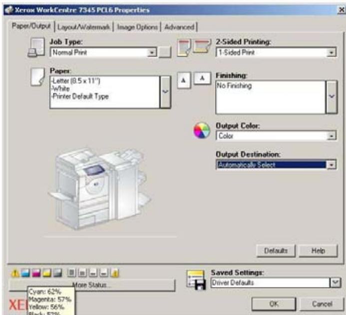
The PCL driver's first tab, Paper Output, provides basic job settings, such as paper size and type, simplex/duplex, document finishing, and color/black-and-white.
