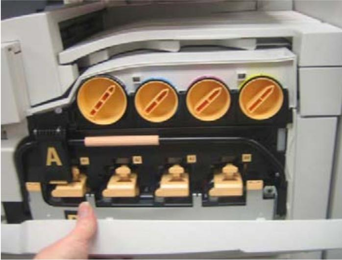
In order to access toner cartridges, drum cartridges and the waste-toner container, the user opens the WorkCentre 7345's front door, as seen above.
