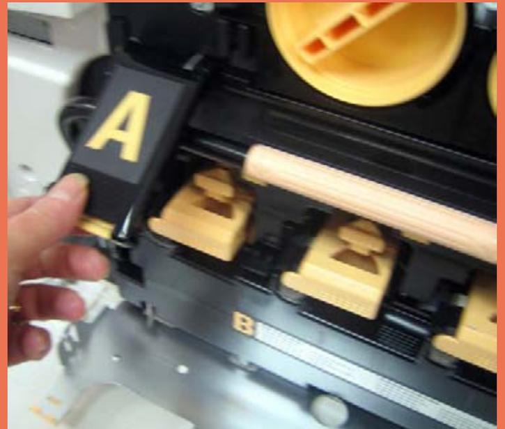
In order to replace the imaging drums and empty the waste-toner container, the user first presses down on the tab labeled "A," then pulls up the handle to the right.
