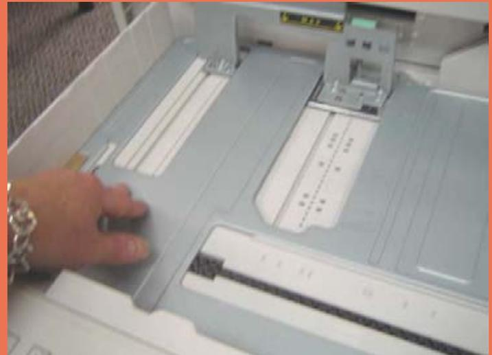
In order to load paper in the bottom drawer, users press down on this plate. Note that whenever a user opens a paper drawer—regardless of whether or not they change the installed paper size—the touch screen prompts them to confirm the installed paper sizes in all paper drawers.
