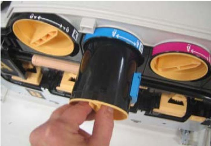
In order to remove one of the four color-coded toner cartridges, the user first unlocks the toner cartridge as seen above.
