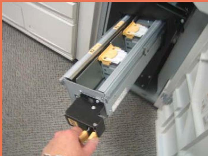
This portion of the finisher may be pulled out for easier access to misfeeds.
