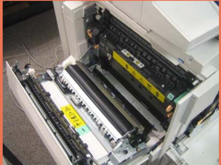
The main misfeed access area on the left side of the device. The touch screen provides explicit instructions for accessing and removing any misfeeds that may occur.
