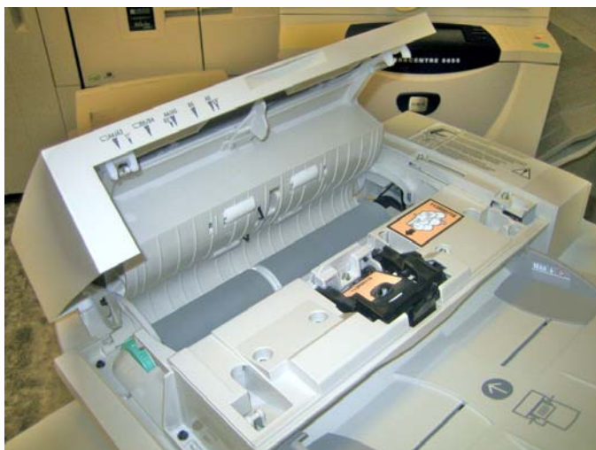
The WorkCentre 5655's document feeder and document-feeder misfeed access.
