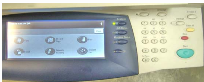
The WorkCentre 5655's Control Panel consists of a touch screen and hard keys.
