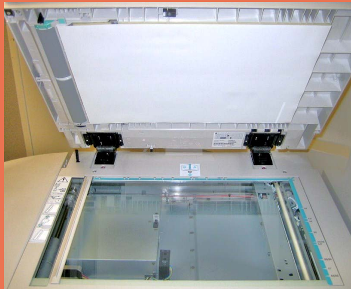
Above and below: The WorkCentre 5655's platen (above) and document feeder (below). The document feeder's cover can be opened for easy access to any misfeeds.
