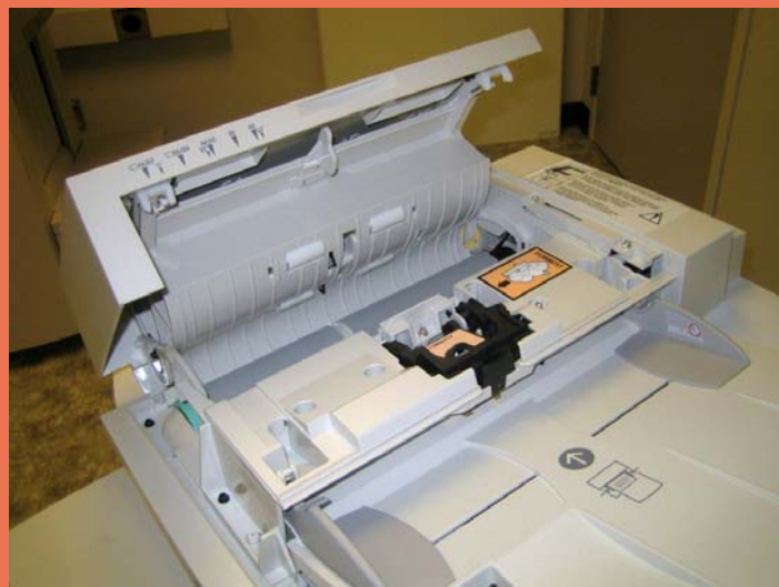
Above and below: The WorkCentre 5655's platen (above) and document feeder (below). The document feeder's cover can be opened for easy access to any misfeeds.
