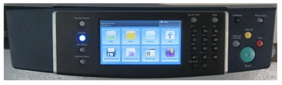
The control panel, which is fixed and can't be tilted, has hard keys, including an alphanumeric keypad, and some LEDs. The Help function offers guidance with specific jobs. Users can check consumables levels by pressing the Machine Status hard key and then the Supplies tab..
