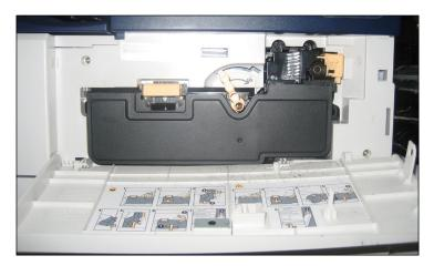
Replacing toner is clean. Note that the side panel of the unit must be opened before the front door can be opened to access toner. A lever in the center of the panel must be rotated to unlock the toner before the cartridge can be removed by pulling the handle
