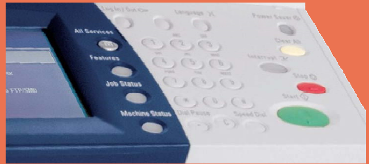
The right side of the control panel contains various hard keys, including keys for "Start," "Stop," etc. as well as a numerical keypad for entering number of copies and fax numbers, keys for switching between different functions (copy, scan, fax, etc.), and hard keys for displaying job status and machine status.
