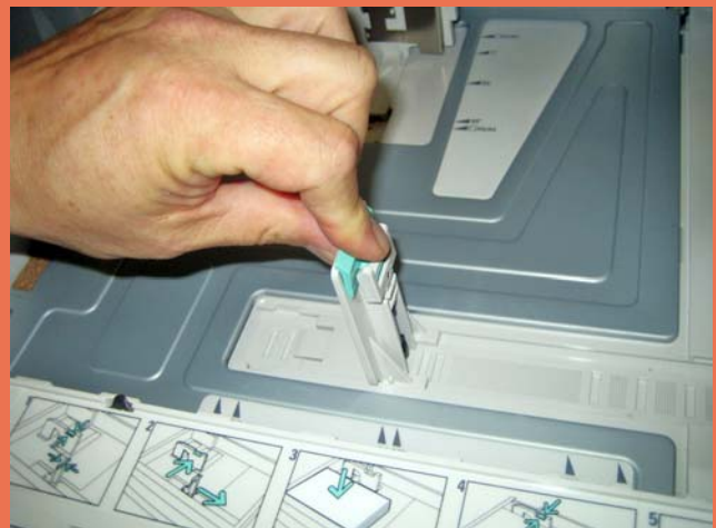
This paper tray is equipped with an end stop that the user must slide in order to adjust the paper drawer to accommodate the desired paper size. Overall, BERTL found adding paper and adjusting paper drawers to be relatively easy.
