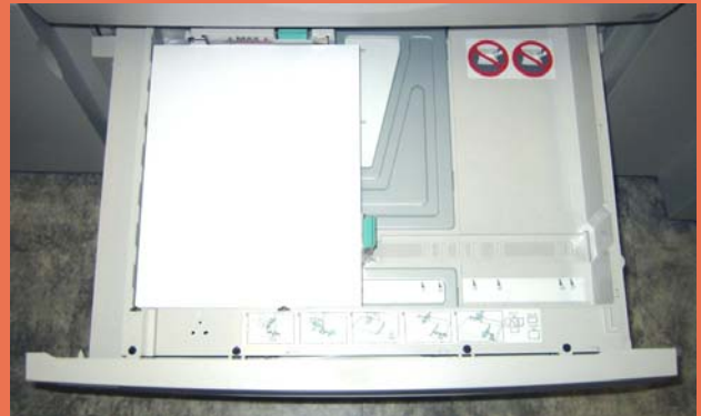
Both the standard tray 1 and optional tray 2 can each hold 520 sheets of 20 lb./80 gsm media (in from 5.5"x8.5"/A5 up to 11"X17"/A3).
