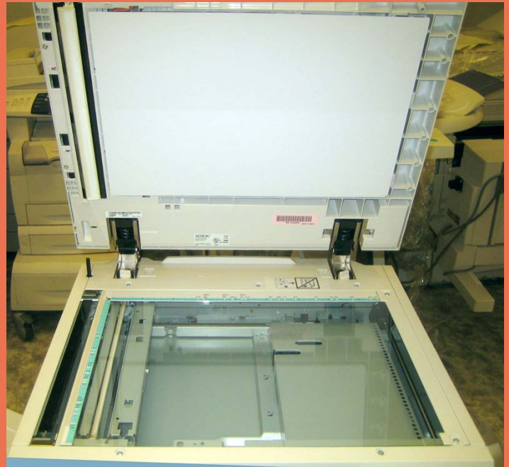
Above and below: The WorkCentre 7242's platen (above) and document feeder (below), with the document feeder's cover opened in order to expose the feeder's misfeed-access area.
