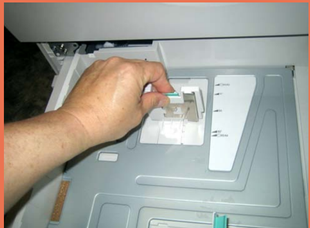
In order to adjust the paper drawers, the user squeezes this green lever and then slides the guide into place.
