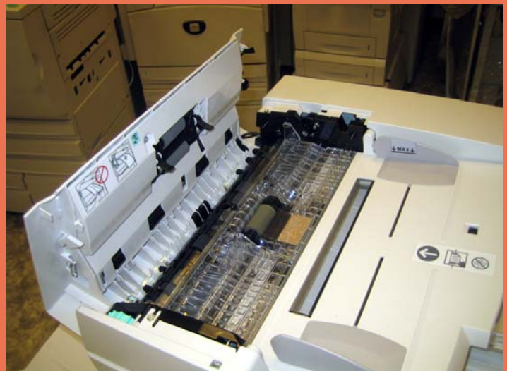
Above and below: The WorkCentre 7242's platen (above) and document feeder (below), with the document feeder's cover opened in order to expose the feeder's misfeed-access area.
