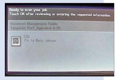
The user then loads the documents to be scanned in the document feeder on the MFP and presses the green "Start" button on the device. The scanned images are then sent.
