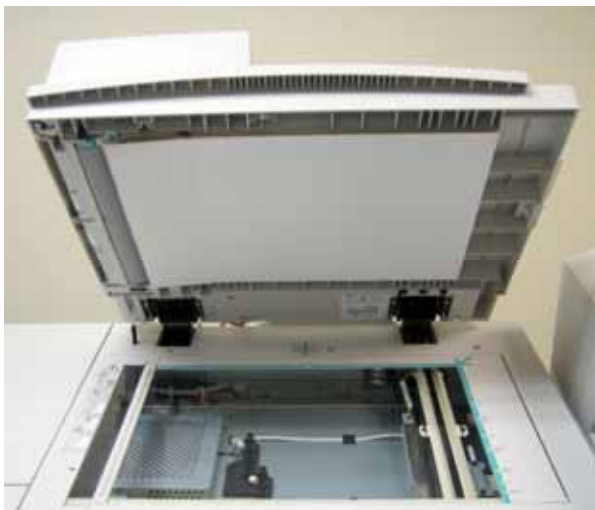
Above and below: The Xerox ColorQube 9203 platen glass and duplex automatic document feeder (DADF).
