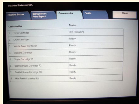
The Machine Status hard key allows the user to view the status of each paper drawer, machine information, billing meter/ print reports and consumables status.
