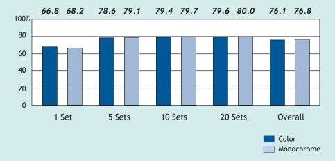
BLI obtains the overall efficiency percentage by dividing the tested speed of the device by the rated speed and then multiplying by 100 for each run length. All jobs are based on a 10-page document printed in the default Enhanced mode using the PostScript driver.
