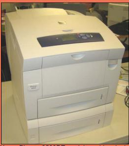
The Xerox Phaser 8560DT model provides duplexing, 512 MB of memory, and an additional 525-sheet paper drawer.
