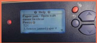
A flashing red LED on the control panel alerts users that the printer is in need of attention.
