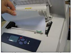
Most paper misfeeds can be easily removed from the front or near the top of the device. BERTL analysts did not encounter any problems or any hidden misfeed points.
