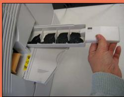
Most minor maintenance requirements for the Xerox Phaser 8560 can be performed in a matter of minutes including emptying the solid-ink waste tray, which is performed when a message appears on the control panel informing users that the waste tray is full.
