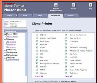
The ability to clone printer settings to be used to configure other printers within the office space will provide a common set of printer settings, which will be a time and resource saver.
