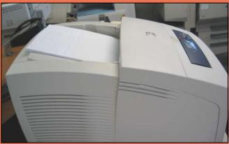
Print jobs are neatly output to the center default tray, providing a base for users to set up collated sets for post-process imposition such as saddle-stitch booklets or perfect binding.
