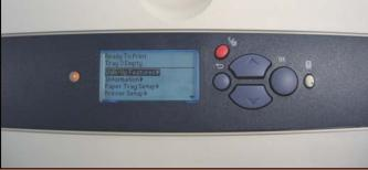
The Phaser 8560's control panel provides an intuitive, walk-through menu system that is relatively easy to use. Navigating through the screens is simple: users press the up and down arrows to move between menus, select the OK button to accept the choice, and then press the return button to exit the specific screen. To cancel a print job currently printing, users can press the red "C" button.
