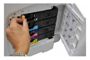
Above and next page: Once the door is open the user then unlocks the orange lever by sliding it to the right and pulling the toner cartridge out for replacement. Overall, BERTL found replacing the all four toner cartridges to be a simple process.
