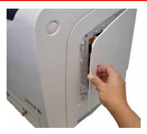
In order to replace the Xerox Phaser 6140N's toner cartridge the user must first open the devices side cover by pulling this panel door open.
