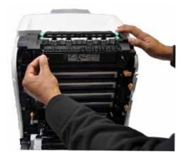
Misfeeds can be cleared in the fuser unit by pulling these two green levers down and removing any jammed paper.
