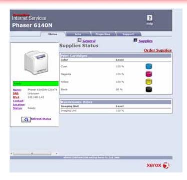
Users can view levels of print cartridges as well as levels of the imaging unit.
