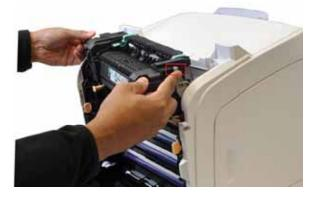
**Above and next column:** In order to replace the fuser unit the users presses this gray lever and slides the unit out for replacement.
