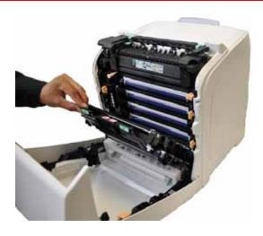
The front misfeed area, feed roller kit and imaging unit can be accessed by lowering the transfer belt unit to clear any jams or replace rollers.
